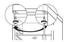
Remove the door handles. To do this, use a screwdriver to turn the rotating pin 1/4 of a turn clockwise and remove.
